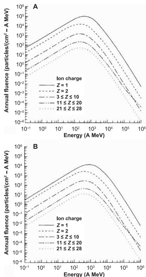
**FIG. 2.** Differential annual fluence spectra. Panel A: GCR ion fluence for 1977 solar minimum. Panel B: GCR ion fluence for 1981 solar maximum. Here energy has been multiplied by atomic number,  $A$ , rather than expressed as  $E/n$ . Note overall reduction in fluence but increase in energy of fluence maximum for solar max. Reproduced and used with permission from Fig. 1 of Wilson *et al.* (37).
