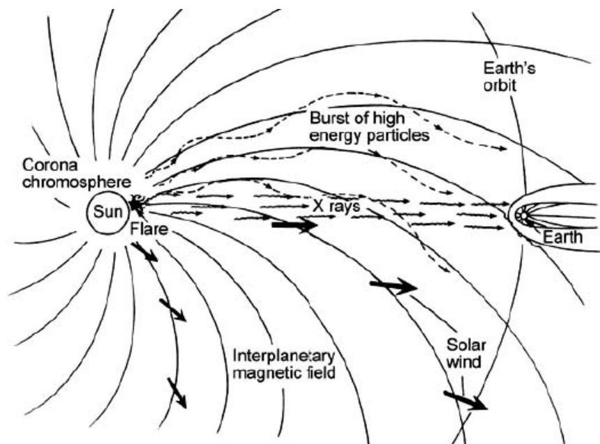
**FIG. 3.** Interplanetary magnetic field, as originating in the Sun and as deformed by the effects of the solar rotation and solar wind. Reproduced and used with permission from Fig. 3.15, NCRP Report No. 153 (7).
