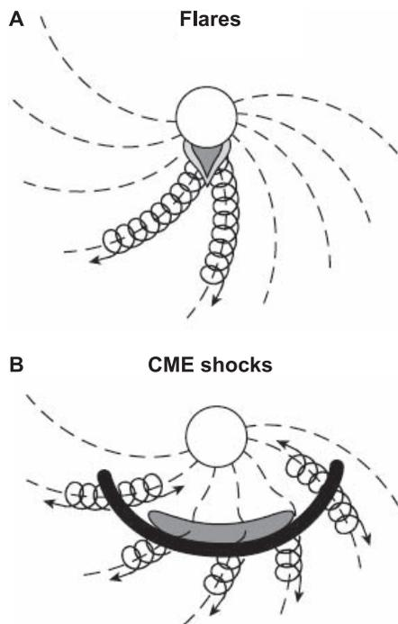
**FIG. 4.** Panel A shows the propagation paths of impulsive SPEs following the Parker spiral field lines, while panel B shows the wide angular dependence of CMEs. Reproduced and used with permission from Fig. 2.1 of Reames (13).
