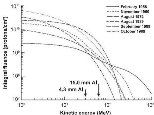
**FIG. 5.** Large SPE integral fluence (sum of all fluence below an energy value) spectra at 1 au. Arrows indicate ranges in aluminum for protons of energy 30 and 60 MeV/n. For these events, total fluence for energies  $>30$  MeV ranged from  $2 \times 10^8$  to  $8 \times 10^9$ . Modified and used with permission from Fig. 3 of Wilson *et al.* (38).
